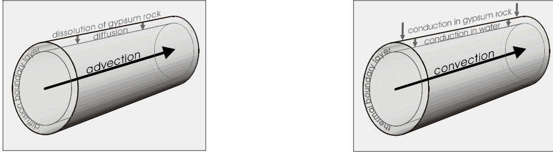
Fig. 1: Mass transfer (left) and heat transport processes (right) in gypsum karst conduits
